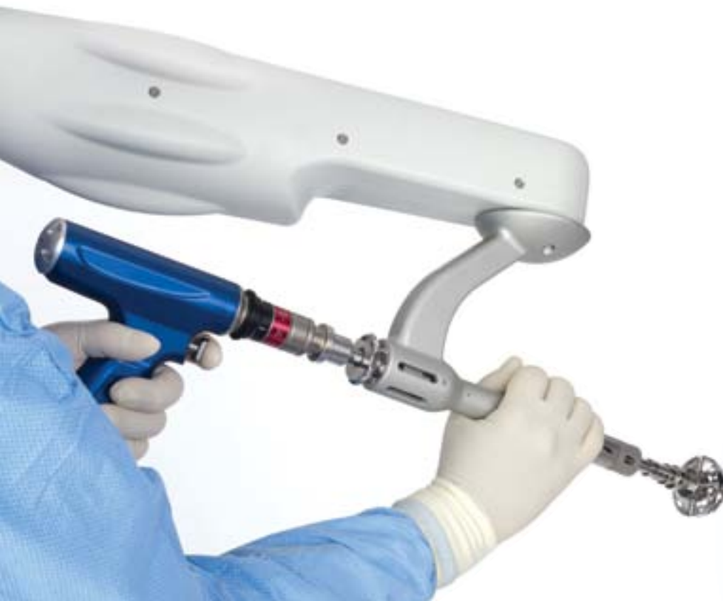
Precision sculpting of bone with RIO® robotic arm
